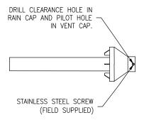
Figure 21. Rain Cap to Small Vent Pipe Ass'y
