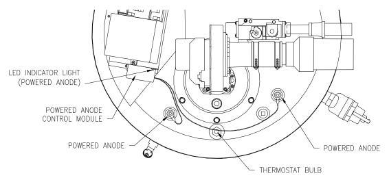
Figure 28. Powered Anode locations
