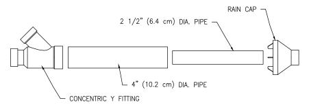
Figure 20. Concentric Vent Kit Part Identification
