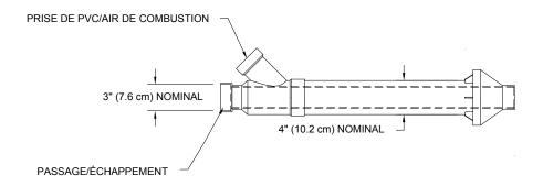
Figure 19. Dimensional Layout of Concentric Vent Kit
