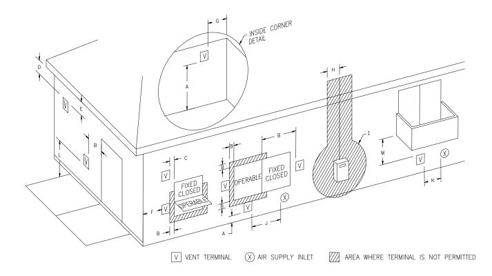
Figure 12b. Direct Vent Terminal Clearances
