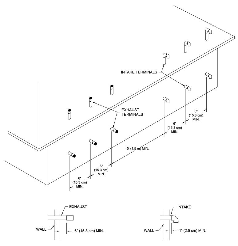
Note: When installing multiple intake/exhaust terminals on the same wall of a building, the nearest intake terminal must be at least 5 feet (1.5 m) from the nearest exhaust terminal. Spacing requirements are the same for roof installation.
