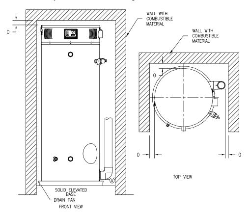
Figure 3a. Minimum Clearance To Combustible Material
