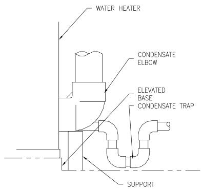
Figure 2. Condensate Elbow with Trap
