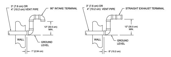
Figure 15. Vent Terminal (Low Ground Clearance)
