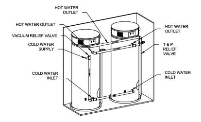
Figure 6. Typical Two Water Heater Connection
