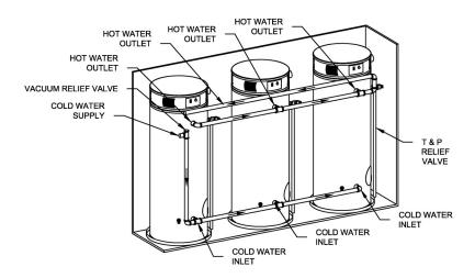
Figure 7. Typical Three Water Heater Connection
