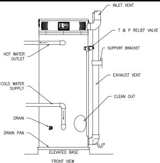
Figure 4. Typical Front Inlet Connection
