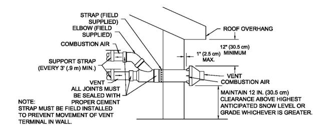
Figure 23a. Concentric Vent Side Wall Attachment
