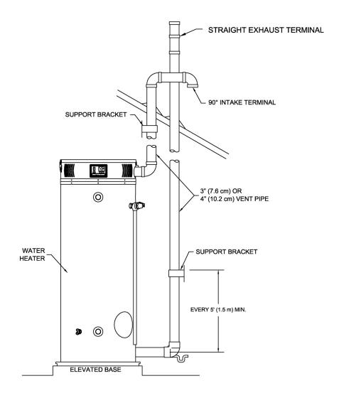
Figure 14. Typical Vertical Direct Vent System Installation
