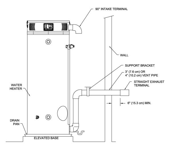
Figure 16. Typical Horizontal Power Vent System
