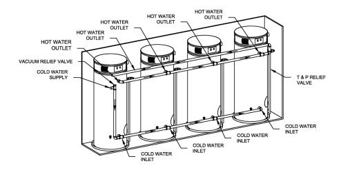
Figure 8. Typical Four Water Heater Connection
