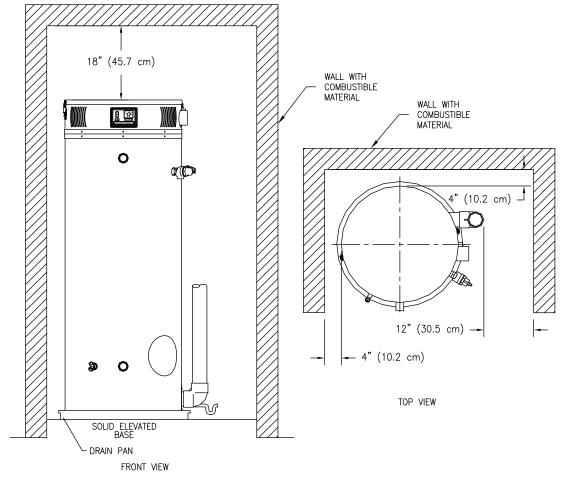
Figure 3b. Recommended Minimum Clearances For Service Access
