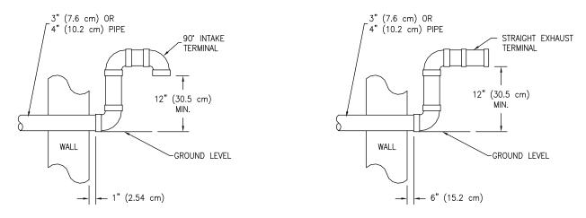
Figure 18. Vent Terminal (Low Ground Clearance)
