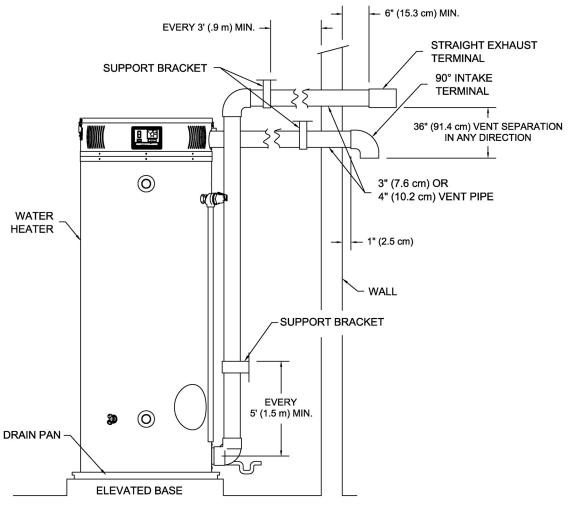
Figure 13. Typical Horizontal Direct Vent System
