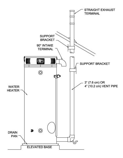
Figure 17. Typical Vertical Power Vent System Installation
