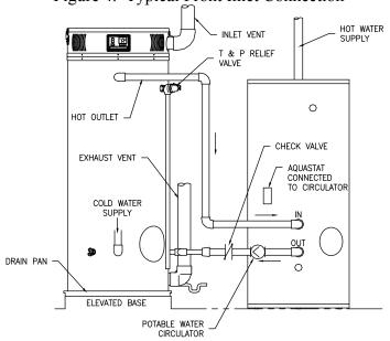
Figure 5. Typical Front Inlet Connect with Storage Heater
