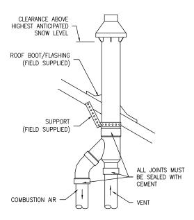
Figure 22. Concentric Vent Roof Top Attachment
