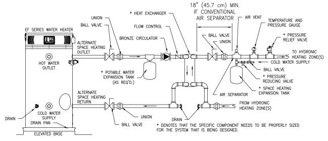
Figure 11. Typical Plumbing Schematic for Zoned Heating
