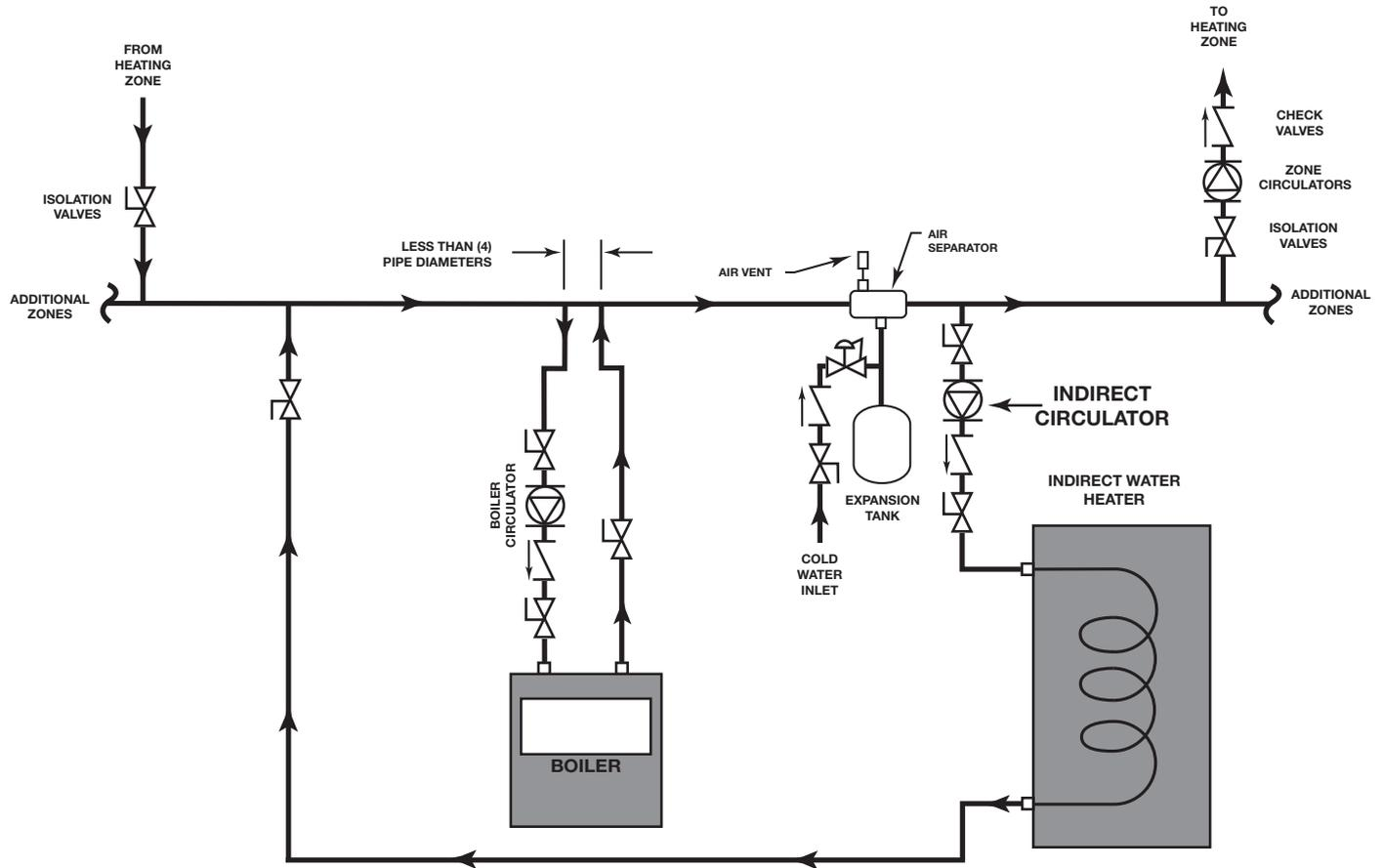
Figure 8: Bock Indirect with Low-Mass Boiler
