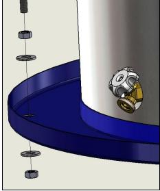
Figure 4: Hardware order of installation
